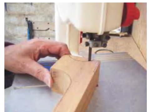
▲ Pic.17 Cutting the 'slipper' on the bandsaw
